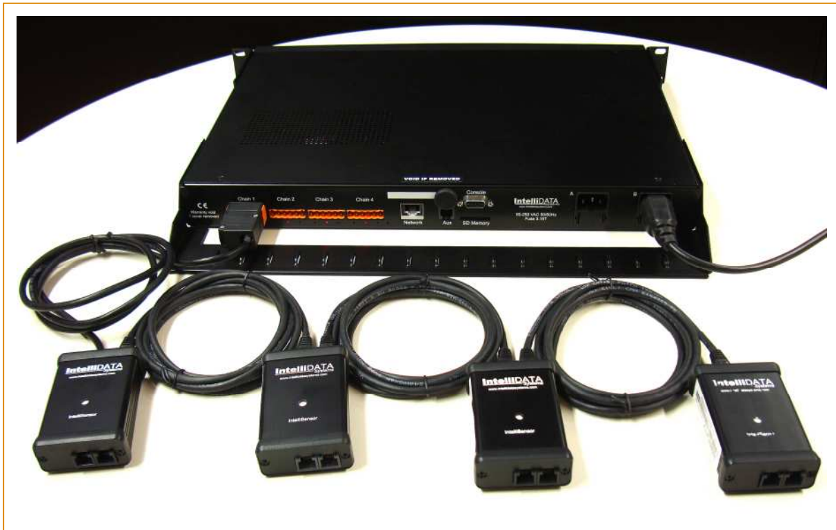
Four IntelliSensors, each providing Temperature and Humidity measurement and two sets of open-door detection connected to 1 chain of an IntelliPoller.
