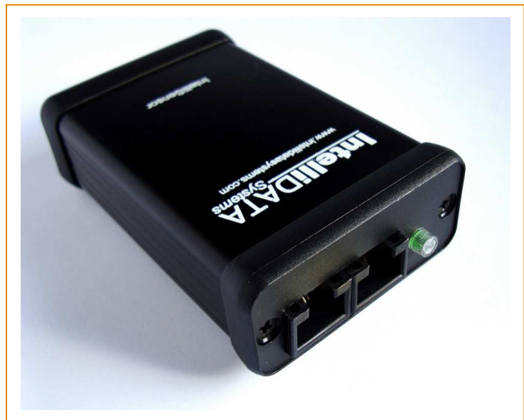
Typical IntelliSensor Showing daisy-chain Serial RJ45 connectors
